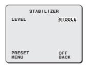
Set [STABILIZER] to "OFF" in the OPTION screen when the correction of the sway is not required.
